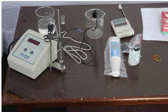
1 Water test kit PH meter, DO meter, Thermometer and ammonia kit
